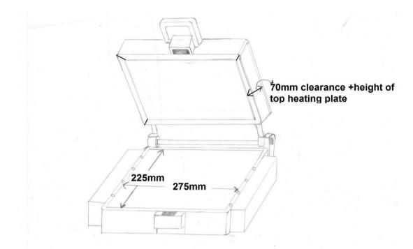
Schematic of the soldering reflow chamber with important dimensions
