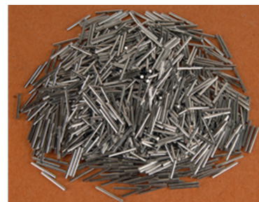
Fig. 13 (a) A prototype stent-graft made by stitching NiTi stent rings on to polyester/dacron cloth; superelastic NiTi stent rings were fabricated at CSIR-NAL, (b) electropolished SE NiTi SMA samples prepared at CSIR-NAL and provided to SCTIMST for biocompatibility and toxicology studies.
