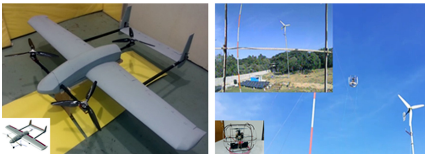
Fig. 8 Design and development of 7 kg VTOL UAV and flight testing of 1 kg VTOL UAV.
