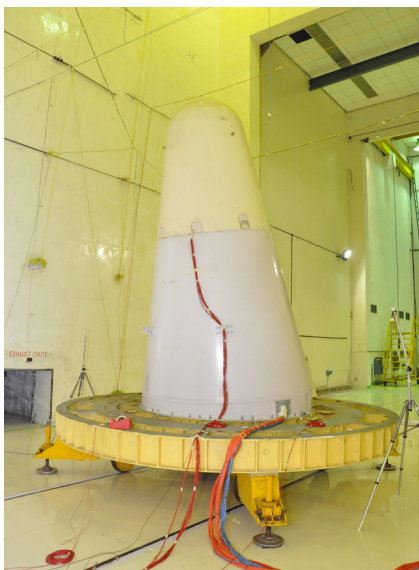
Fig. 12 GSLV-L40 SONC acoustic test.
