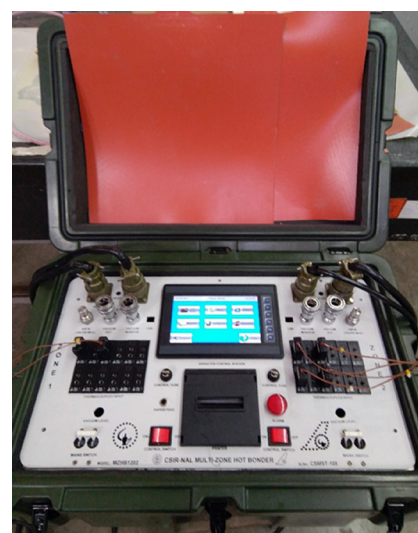
Fig. 10 Multi zone hot bonder with 12 heater control.
