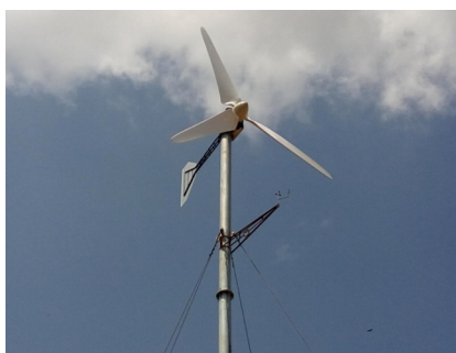
Fig. 15 4 kW NALWIN Wind Turbine. will be installed at the CSIR-IMMT campus at Bhubaneshwar under the CSIR-800 banner program. Under the FTT programme, NAL has taken up design and development of 4kW and 10 kW WiSH system for low wind regimes prevalent across the Indian subcontinent. The 4 kW hybrid is designed to deliver 4 kW at least 8 hours a day and the 10 kW system is designed to address the energy demand of off-grid rural populace at community level. The installation of hybrid system are in progress at NAL (4-10 kW) and at KREDL (10-15 kW), Nagarabhavi, Bengaluru (Fig. 15). I am also happy to inform that the fourth order for lab scale autoclave was received from IIT- Bombay during the year.
