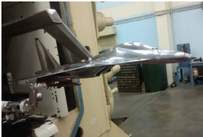
Fig. 10 A photograph of the model along with parent aircraft mounted in the 1.2m tunnel.
