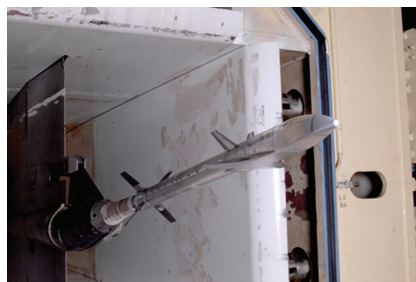
Fig. 12 A photograph of RLV ascent phase model mounted in the 1.2m tunnel.
