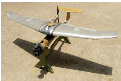
Fig. 4a SUCHAN UAV with 2m wing span.
