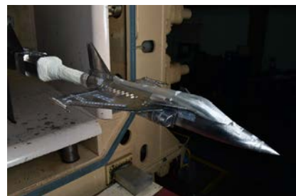
Fig. 16 A photograph of typical combat aircraft model mounted in 1.2m tunnel.
