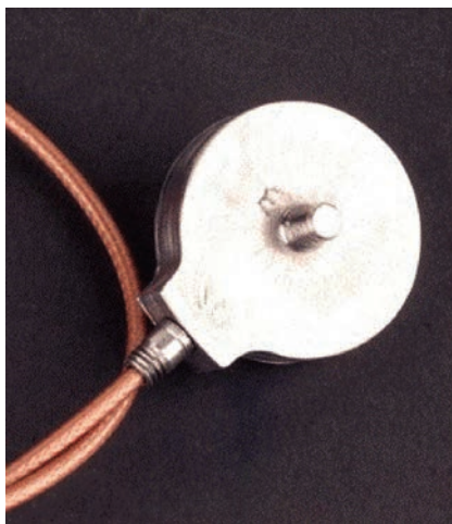
Fig. 15 Photograph of PE accelerometer with stud mount configuration.
