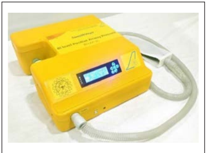
Fig. 2 SwasthVayu - BiPAP Non-invasive Ventilator.
