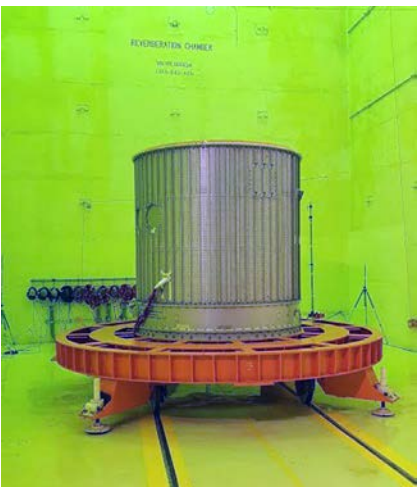
Fig. 20 Test vehicle inter tank structure with EB.
