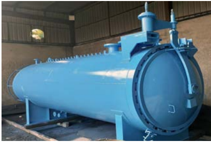
Fig. 7 Industrial grade Autoclave fabricated by ToT Partner M/s. KRR Engg, Chennai for M/s. BEL, Bengaluru.
