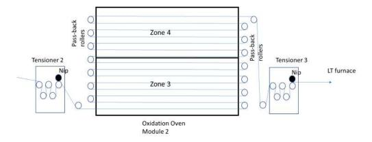
**Fig.4** Representation of Stabilization Oven - Module 2
