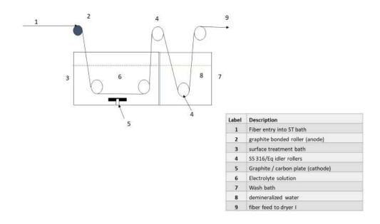
As the (DC) current passes through the bath solution, the fibers get oxidized by virtue of being in contact with the anode. The extent of oxidation is controlled by adjusting the bath current. The electrical contacts with the anodic rollers are to be established through suitable commutator rings.
