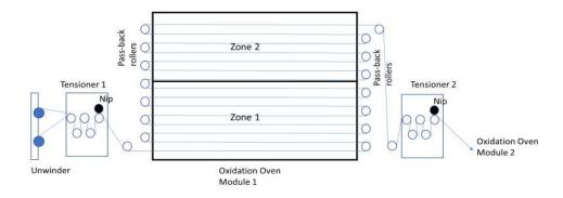
Fig.3 Representation of Stabilization Oven module 1
