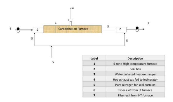
Fig.6 Schematic representation of the carbonization furnace
