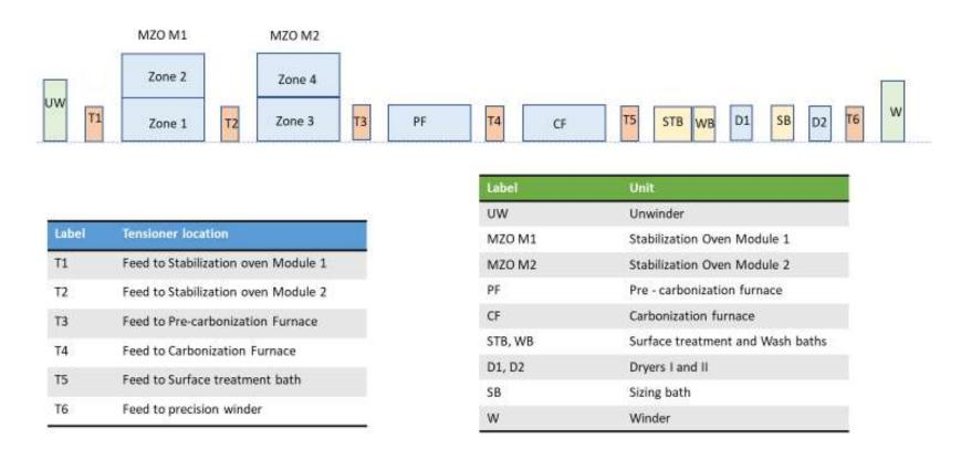
Fig.2 Schematic configuration of the equipment units in the heat treatment line
