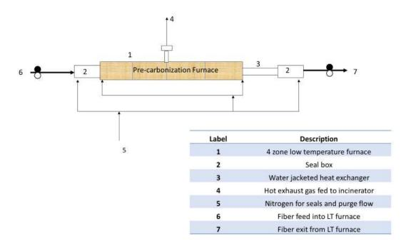
Fig.5 Schematic representation of Pre-carbonization furnace
