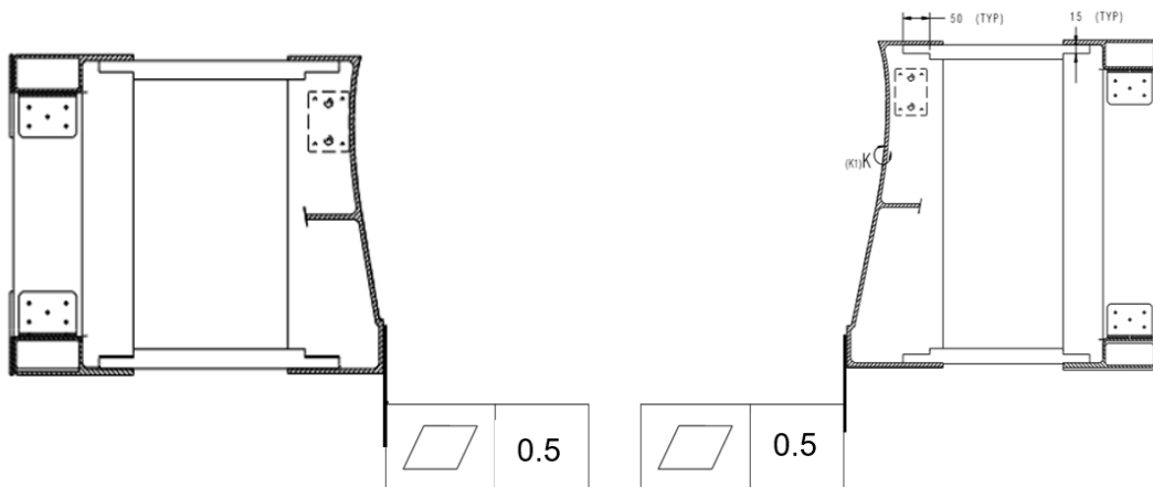
Figure 8. Flap Aft Box sections at Root & Tip of the Mould (LH)
