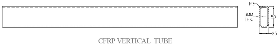
Figure 3. CFRP Vertical Tube (Rectangular Tube) with Dimensions
