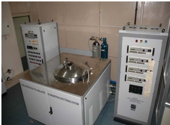
Semi-industrial sputtering facility
