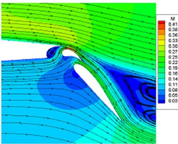
Fig. 7. Mach Contours and Stream Lines Plot for NACA 1410 double slotted airfoil.
