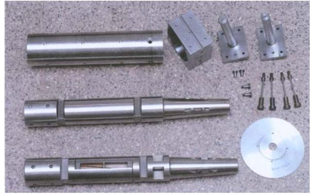
Fig. 15. 2.5" In-house designed integral balances and components.
