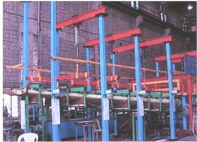
Fig. 5. Saras wing load testing.
