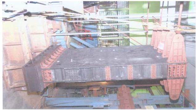
Fig. 1. Wing test box under static test.
