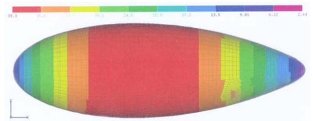
Fig. 18. Hoop stress distribution in the hull for an internal pressure loading.
