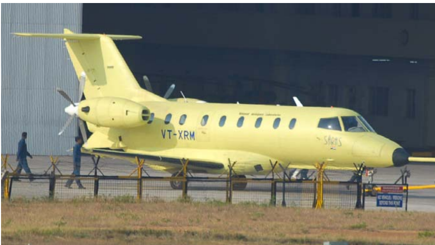
↓ Fig. 1 SARAS PT2 - the second prototype of the 14 seater light transport aircraft.
