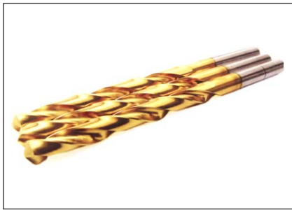
↑ Fig. 15 Nano-structured TiN coated HSS drill-bits.
