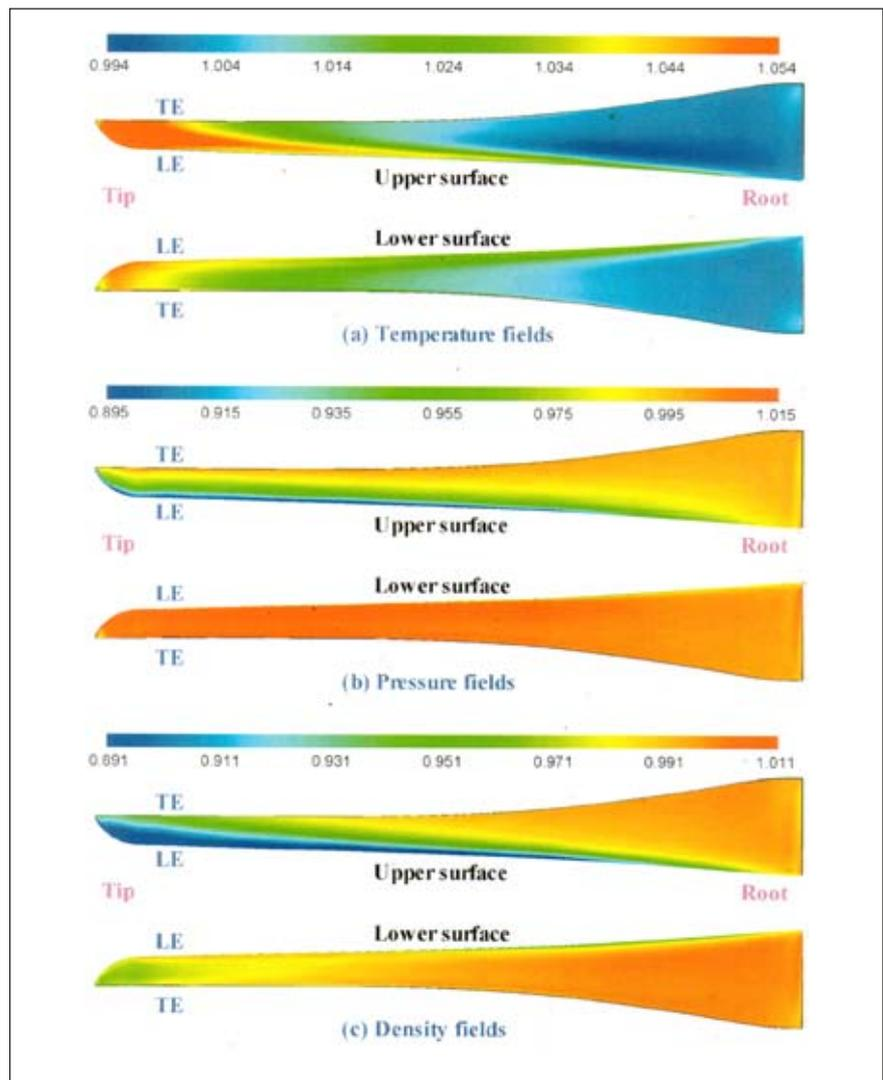
↑ Fig. 5 A detailed CFD analysis is being undertaken for the development of a 500kW low cost horizontal axis wind turbine. The figure shows typical fields of temperature, pressure and density on the upper and lower surfaces of the blade.
