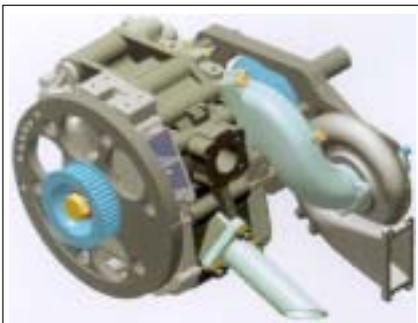
↑ Fig. 10 NAL's Propulsion Division, jointly with VRDE, is designing and developing a 55 hp Wankel rotary engine for unmanned aerial vehicles. The solid model of the core engine is shown in the figure.
