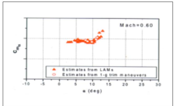
↑ Fig. 7 Typical results from a study at the Flight Mechanics and Control Division to estimate the local pitch-up tendency of an aircraft.
