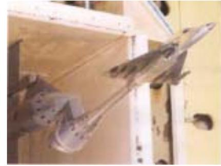
Model mounted on twin roll model support system in the 1.2m tunnel.
