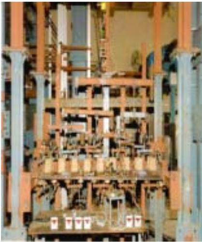
↑ Fig. 2 The Advanced Composites Division has developed composite control surfaces (elevators, ailerons, rudder and flaps) for the SARAS aircraft. The photograph shows the cyclic load test being carried out on the SARAS outboard flap.
