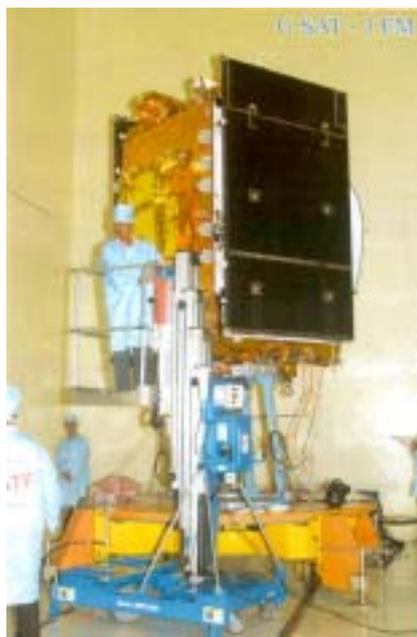
↑ Fig. 3 GSAT-3 (FM) spacecraft getting ready for acoustic test in the 1100 cu m reverberation chamber.
