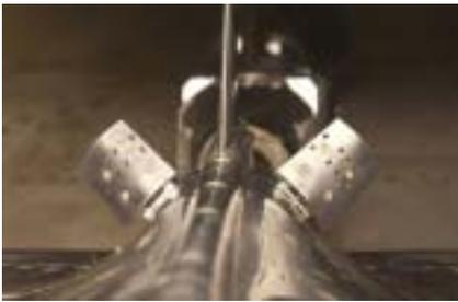
↑ Fig. 9 Wind tunnel tests were undertaken at NTAFA on Tejas airbrake performance studies. NAL's wind tunnels continue to be very valuable for all national aerospace programmes; the tunnel's performance and efficiency will improve even more after the current augmentation exercise ends.
