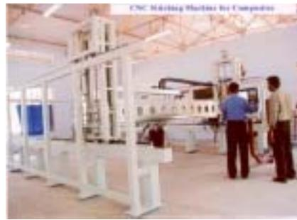
CNC stitching machine for composite structures
