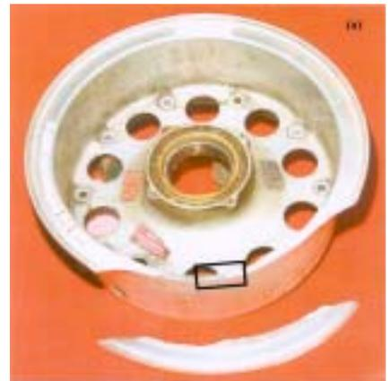
⇔ ↓ Figure 11: The fractured wheel hub of an aircraft and the fatigue crack origin.
