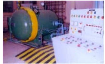
↑ Figure 11 The re-commissioned devine autoclave. Practically the entire autoclave, except the main shell, had to be redesigned and rebuilt.
