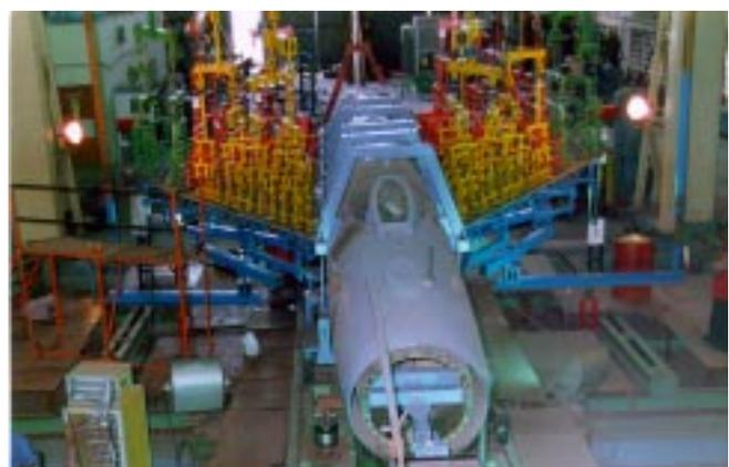
5. LCA Composite Wing Box Test / Dr B K Parida
