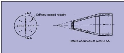
↑ **Figure 4** The Experimental Aerodynamics Division has developed a software package for the calculation of flight parameters for use in a flush air data system. The figure shows the schematic of a typical flush air data probe.
