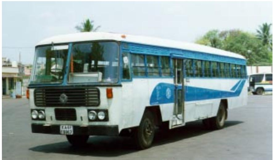
↑ **Figure 5** A KSRTC bus modified to minimize aerodynamic drag. The initial field trials of the prototype buses have yielded encouraging results in terms of fuel savings.
