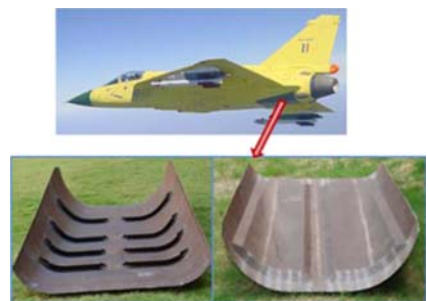
Fig. 6 The Engine Bay door (middle) of LCA using high temperature Carbon/ Bismaliemide prepreg system with a service temperature of 200 deg C.
