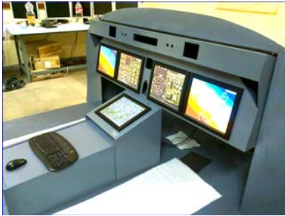
Fig. 21 Integrated advanced display system for regional transport category aircraft avionics.
