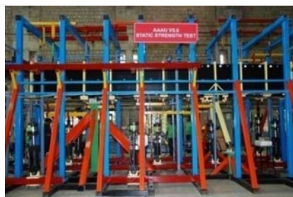
Fig. 11 Static structural strength test setup for AAAU.
