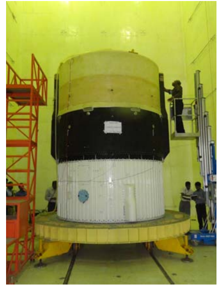
Fig. 15 GSLV CUS inside the RC of ATF.
