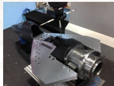
Air force air intake wind tunnel model at Coordinate Measuring Machine
