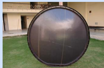
Rear pressure bulkhead for Saras
